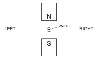
The wire is moved and a current is induced upwards, out of the paper.
